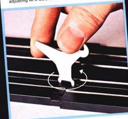
Holding the Quikee-Lok firmly, insert it straight into the track slots. Twist firmly in the direction indicated (counterclockwise) until the track snaps into place.
